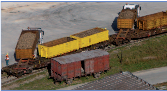
Railcar-container system from the sugar factory 'Sered' in Slovakia
